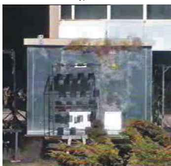
Internal arc type test 20kA/1s
